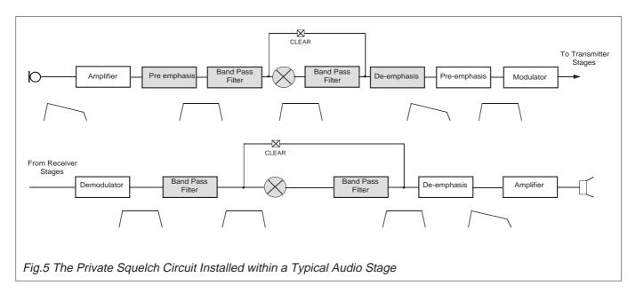
FX375 (shaded areas) when installed within the audio stages of a typical transceiver system. The accompanying waveform diagrams indicate the relative "voice band amplitudes" at each stage of the receive or transmit process.
